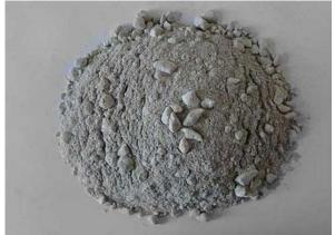
Refractory Cementitious Grout - RCG<sup>™</sup>
