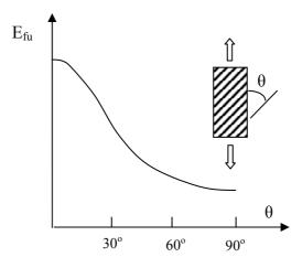
Fig. 5-1: Dependence of FRP elastic modulus on fibre orientation.
