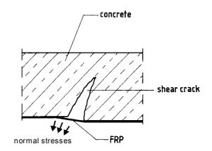
Fig. 4-12: Peeling-off caused at shear cracks.
