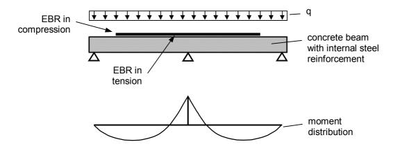
Fig. 4-16: Example of an unintentional use of EBR in compression.
