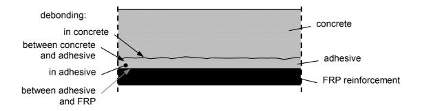
Fig. 4-3: Different interfaces for bond failure.
