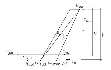
Fig. 3-2: Strain distribution at ULS in the critical section of strengthened flexural members.
