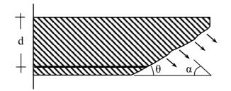
Fig. 5-5: Contribution of FRP to shear capacity.
