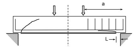
Fig. 4-10: FRP plate-end shear failure.
