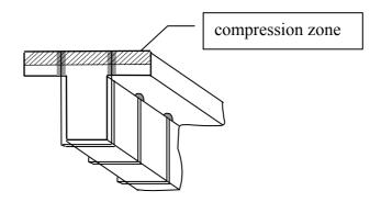
Fig. 7-3: Anchorage in the compression zone.
