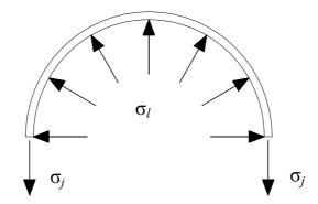
Fig. 6-3: Lateral confining pressure exerted by the jacket.
