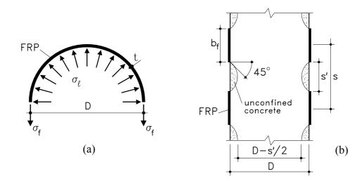
Fig. 6-7: Confining pressure exerted by the FRP.
