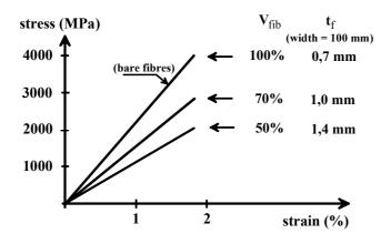
Fig. 2-1: Stress strain relations corresponding to various fibre volume fractions  $V_{fib}$  in Table 2-4.
