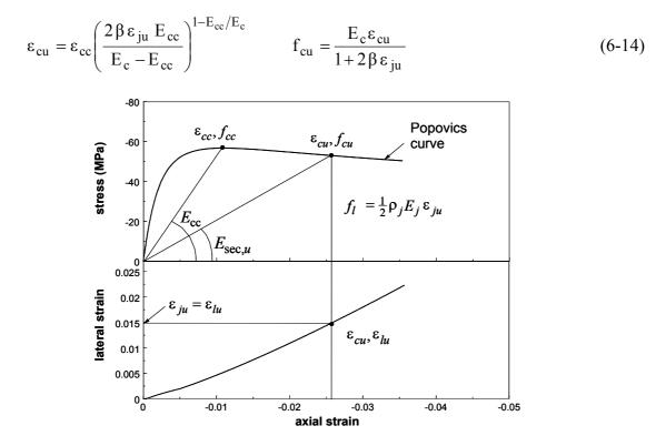
Fig. 6-6: Calculation procedure for ultimate compressive stress and strain.
