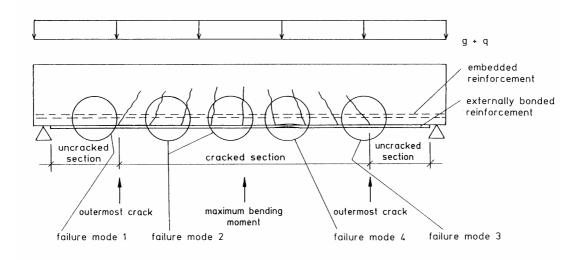
Fig. 4-9: Bond failure modes of a concrete member with EBR (Blaschko et al. 1998).
