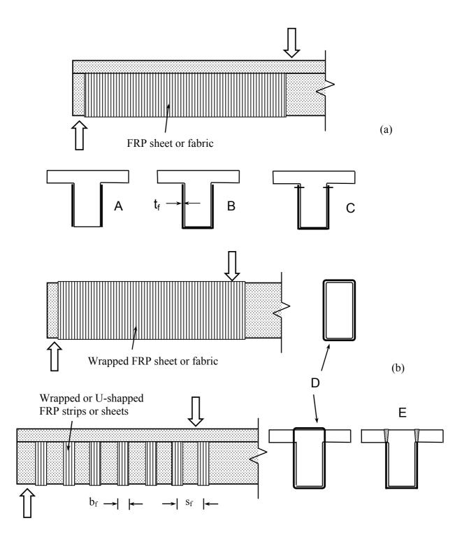
*Fig. 5-2:* Schematic illustration of reinforced concrete element strengthened in shear with FRP: (a) FRP sheets or fabrics bonded to the web; (b) wrapped or U-shaped FRP (the concept shown in D is applicable to both beams and columns).
