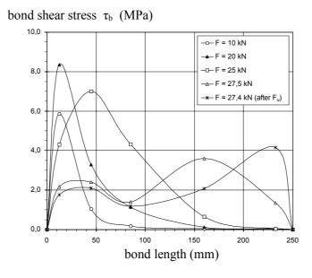
Fig. 4-6: Distribution of shear stresses along the bond length (Zilch et al. 1998).
