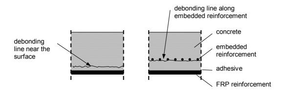
Fig. 4-4: Different debonding lines in the concrete.
