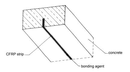
Fig. 2-9: CFRP strips glued into slits.
