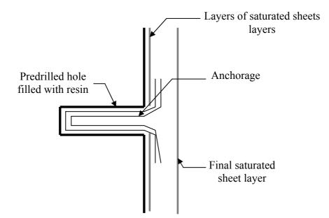
Fig. 7-7: Section of the anchor system.
