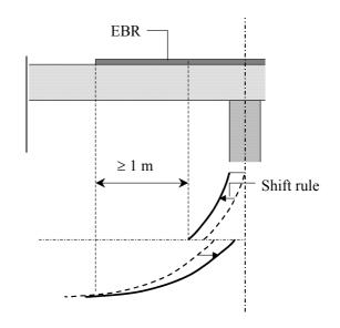
Fig. 7-2: Anchorage above internal supports.
