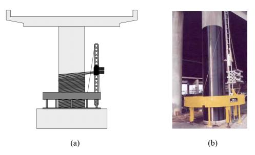
Fig. 2-3: Automated RC column wrapping. (a) Schematic. (b) Photograph of robot-wrapper.
