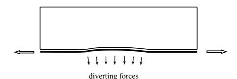
Fig. 4-14: Peeling-off caused by unevenness of concrete surface.
