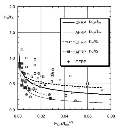
*Fig.* 5-7: Normalized FRP strain in terms of  $E_{fit}\rho_f / f_{cm}^{2/3}$  – shear failure combined with or followed by FRP fracture.
