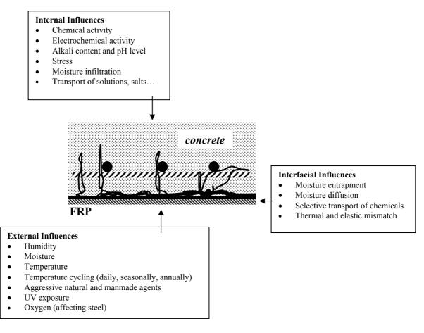
Fig. 9-1: FRP system level interactions.
