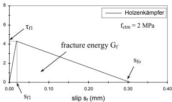
Fig. 4-8: Models for the shear stress - slip relations of EBR (Holzenkämpfer 1994).
