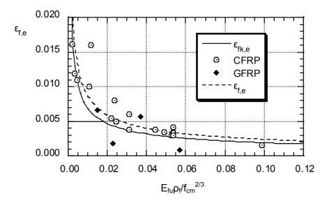
Fig. 5-6: Effective FRP strain in terms of  $E_{fu}\rho_f/f_{cm}^{2/3}$  – shear failure combined with FRP debonding.
