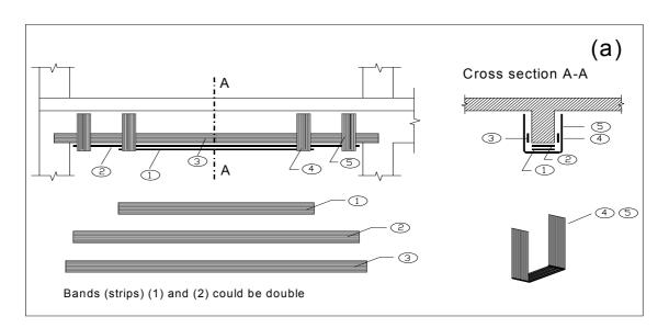
Fig. 7-1: Flexural reinforcement with possible shear anchorages.
