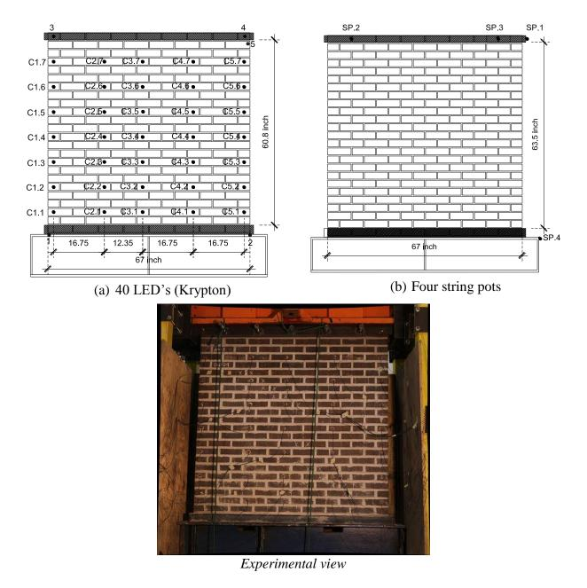
Figure 8-17. Instrumentation of the walls
