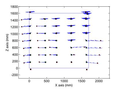
Figure 8-48. Deformation of the wall under cyclic loading (×10)
