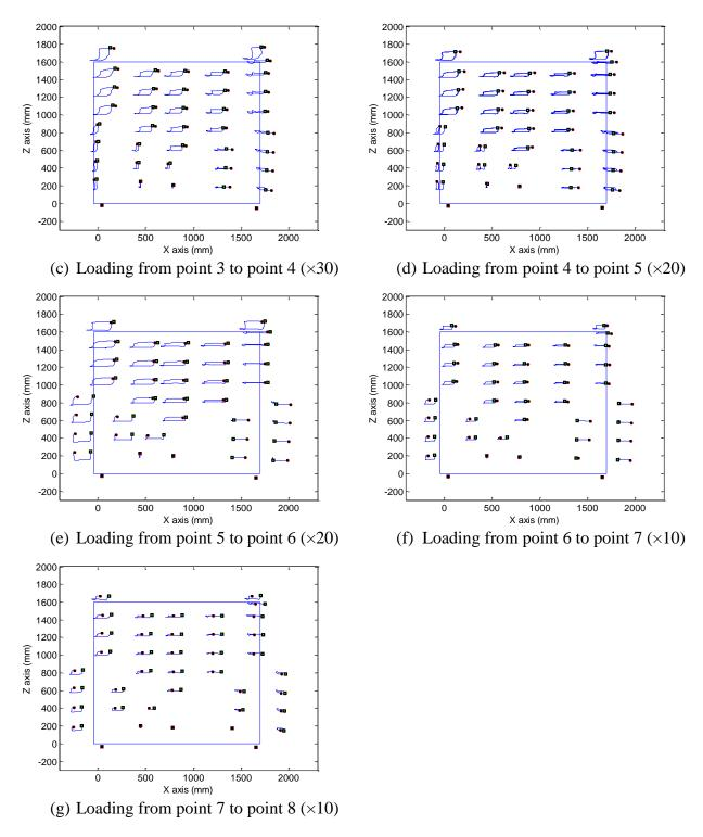
Figure 8-63. Deformation of the wall in different stages of loading
