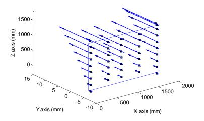
Figure 8-76. Three-dimensional deformation of the wall under OP loading
