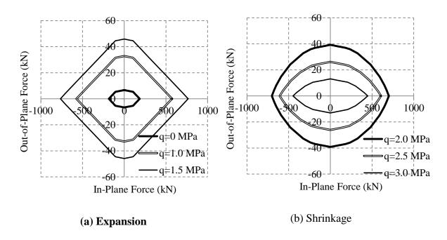
Figure 7-15. Expansion and shrinkage of interaction curve by variation of compressive traction
