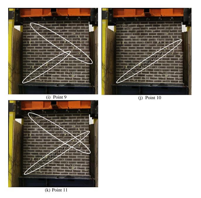
Figure 8-40. Crack propagation of the wall in different stages of loading
