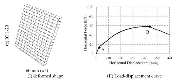
Figure 6-10. Deformed shape and load-displacement for IO:1/10, IO:1/12 and IO:1/20
