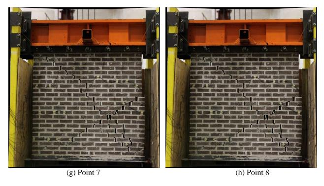
Figure 8-50. Crack propagation of the wall in different stages of loading
