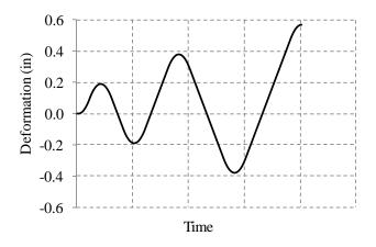
Figure 8-84. Numerical loading protocol
