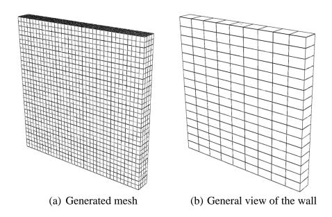
Figure 5-3. Numerical modeling of a masonry wall
