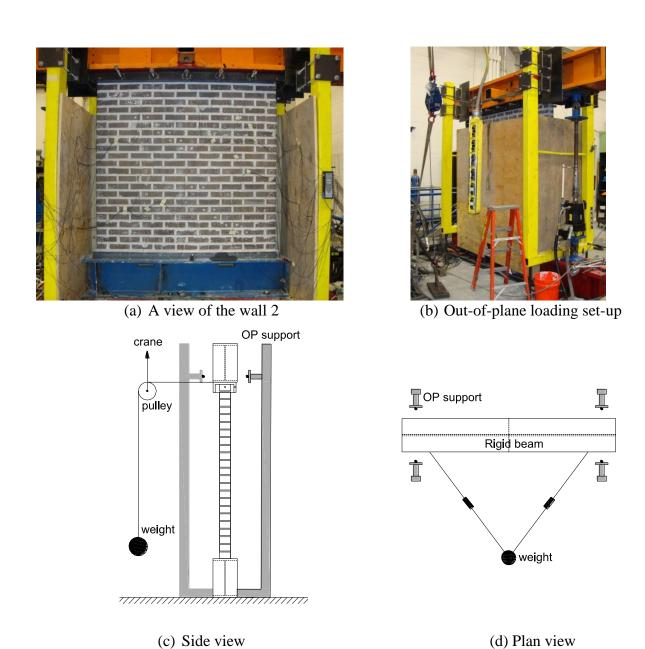
Figure 8-31. Experimental set-up for wall 2
