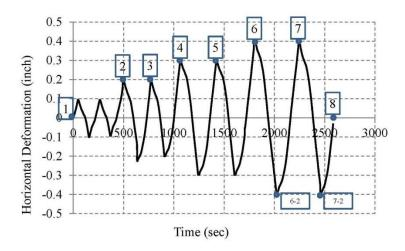
Figure 8-70. Cyclic loading protocol of wall 5
