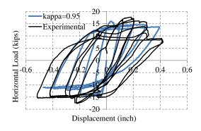
Figure 8-53. Comparison of the experimental and numerical load-displacement curves
