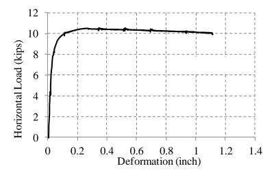
Figure 8-22. Load - displacement of wall 1 (experimental)
