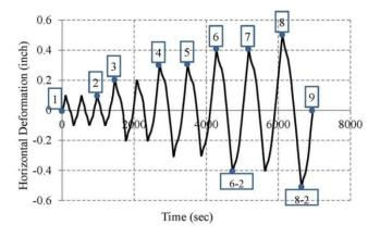
Figure 8-88. Loading protocol for wall 6
