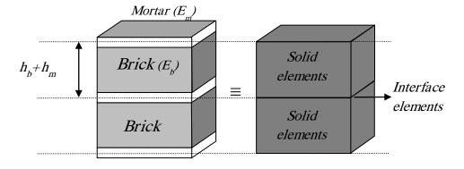
Figure 5-2. Detailed model of brick and mortar
