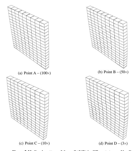
Figure 5-23. Crack pattern of the wall (J6D) in different stages of loading
