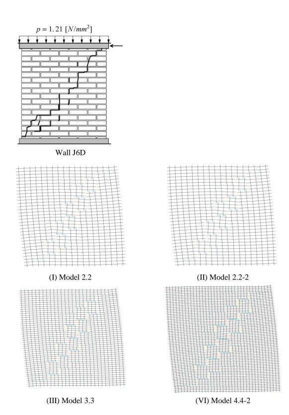
Figure 4-25. Comparison between the cracks obtained by the numerical and experimental models (J6D)
