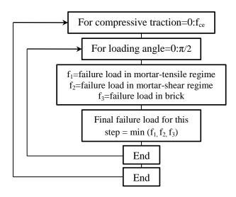
Figure 7-9. Algorithm for the MATLAB code
