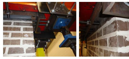
Figure 8-3. Boundary condition for the top plane of the walls
