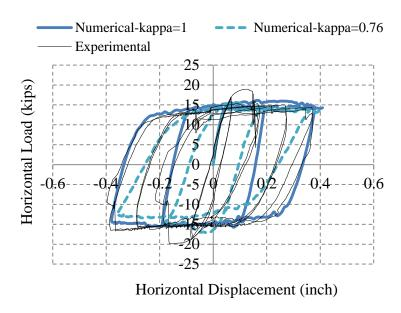
Figure 8-85. Comparison of the numerical and experimental results
