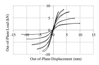
Figure 5-30. Out-of-plane cyclic load-displacement
