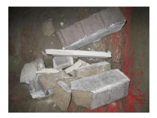
Figure 5-11. The damaged specimen after compression test
