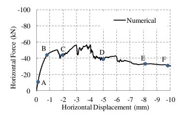
Figure 5-16. Numerical load - displacement result for wall subjected to  $30 \ kN$  compressive load
