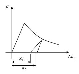
Figure 5-5. Cyclic tensile loading (Oliveira and Lourenco 2004)
