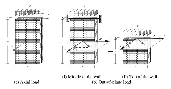
Figure 7-1. A URM shear wall under bidirectional loading
