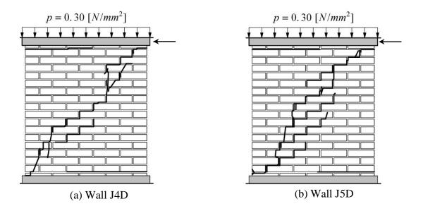
Figure 5-18. Experimental crack pattern at 4 mm displacement (Lourenco 1996)
