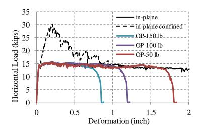
Figure 8-41. Load-displacement curves obtained by the numerical model considering different OP loads
