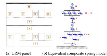
Figure 2-5. Composite spring model of a URM panel (Park et al. 2009)
