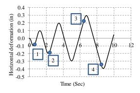
Figure 8-51. Loading-protocol for numerical model
