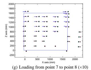
Figure 8-78. Deformation of the wall in different stages of loadings
