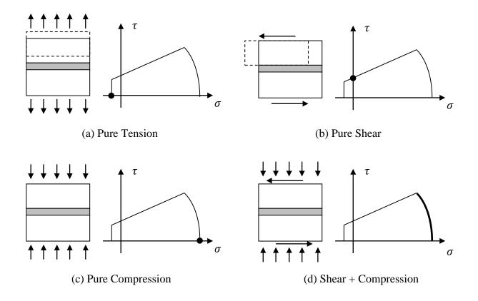
Figure 4-3. State of stress for different types of loadings
