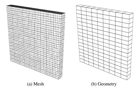
Figure 7-18. (a) General mesh of the wall and (b) General view of the wall
