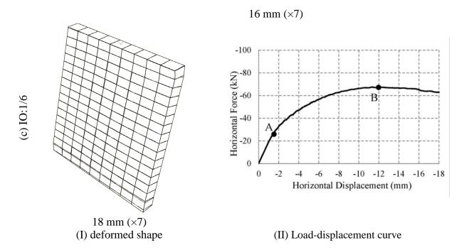
Figure 6-8. Deformed shape and load-displacement for IO: IO:1/4, IO:1/5 and IO:1/6
