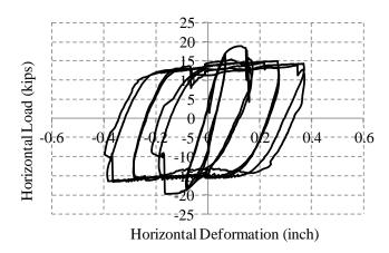
Figure 8-72. In-plane load-displacement using Krypton 5x data
