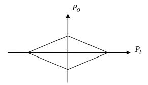
Figure 7-7. Interaction curve governed by tensile failure
