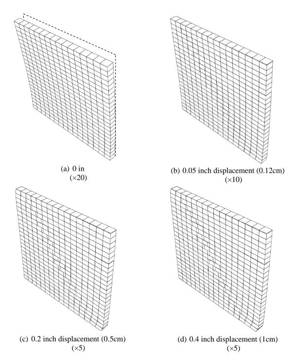
Figure 8-82. Crack propagation obtained from the numerical simulation under monotonic OP/IP loading
