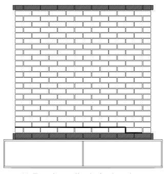
(c) Experimentally obtained crack pattern
