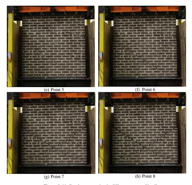
Figure 8-64. Crack propagation in different stages of loading
