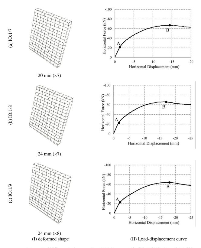
Figure 6-9. Deformed shape and load-displacement for IO:1/7, IO:1/8 and IO:1/9
