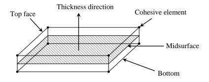
Figure 5-1. Eight node plane interface element (ABAQUS)
