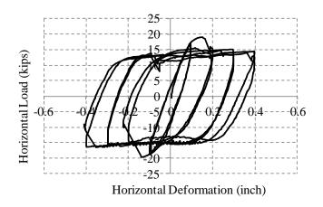
Figure 8-71. In-plane load-displacement of wall 5
