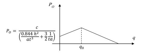
Figure 7-6. Interaction curve for shear-compression
