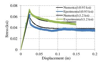
Figure 8-15. Joint behavior under shear displacement considering different confinement pressures
