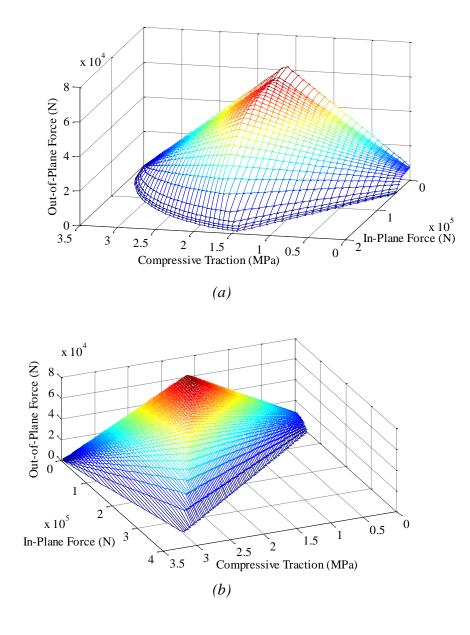
Figure 7-17. Interaction curve for a wide wall (a) including shear failure in the bricks (b) excluding shear failure in the bricks
