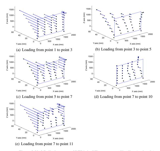
Figure 8-39. 3-D displacement of LED's in different stages of loading (real scale)
