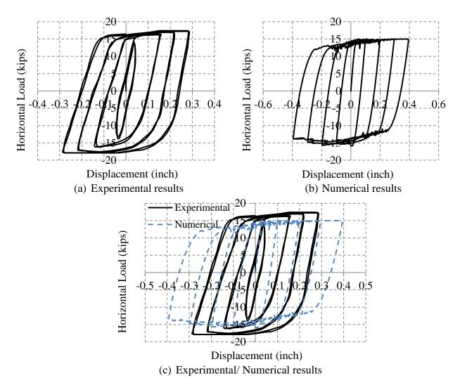
Figure 8-68. Comparison of the numerical and experimental load-displacement curves
