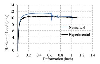
Figure 8-25. Load-displacement curves of the numerical and experimental models. In addition to the numerical comparison, the experimental results could be compared to the empirical formulation presented in ASCE 41 (2006). ASCE 41 predicts the stiffness of cantilever shear walls as follow:
