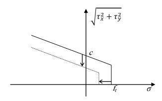
Figure 5-4. Yield surface for the joints
