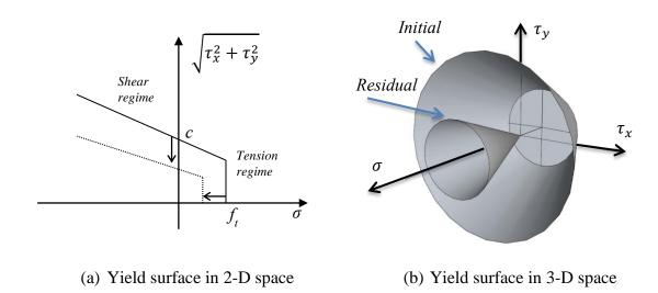
Figure 7-4. Yield surface for the joints
