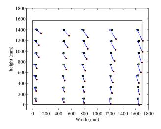
Figure 8-18. Deformation of the wall under the axial load ( $\times$ 500)
