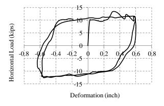
Figure 8-28. Load-displacement curve for cyclic testing of wall 1
