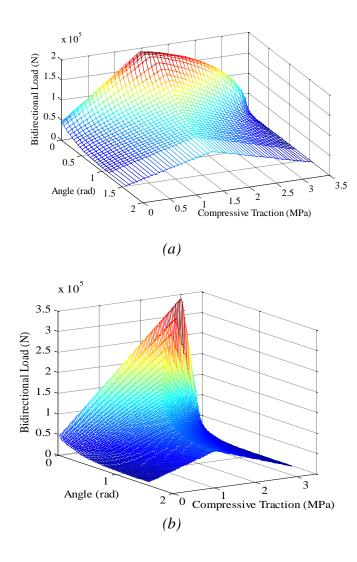
Figure 7-16. Variation of bidirectional load as angle and compressive traction change (a) including shear failure in the bricks (b) excluding shear failure in the bricks
