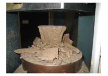
Figure 8-10. A damaged high strength brick after uniaxial compression test
