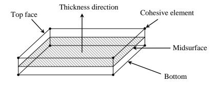
Figure 6-1. Eight node plane interface element (ABAQUS)
