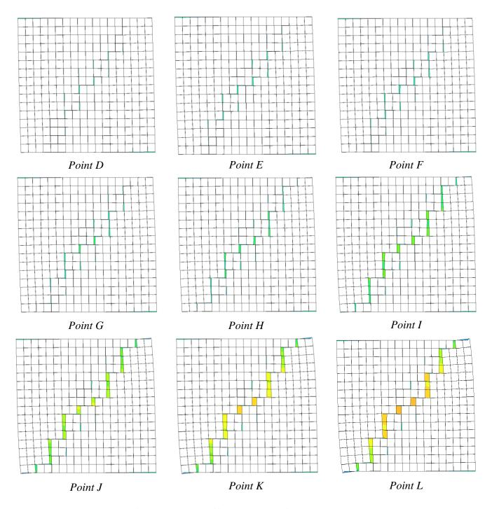
Figure 3-17. Crack path in different stages of loading (Based on the model 4PB-under  $30\ kN$ )
