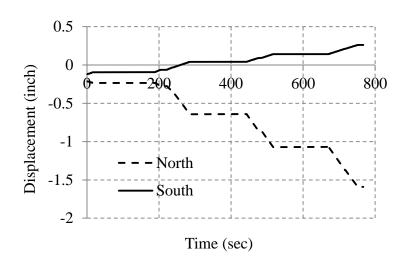
Figure 8-21. Axial displacement of the north and south vertical actuators
