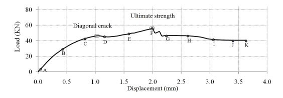
Figure 3-13. Load-displacement graph for J4D and J5D wall (Based on the model 2PB)
