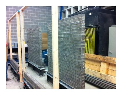
Figure 8-2. Wall type II (the first row of brick is buried into the mortar)
