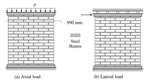
Figure 5-14. Step 1 and step 2 for applying the load (Lourenco 1996)
