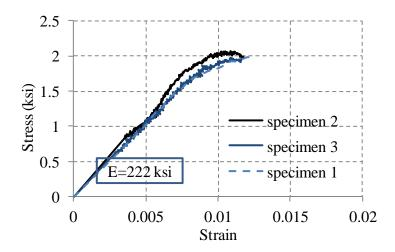
Figure 8-16. Mortar properties
