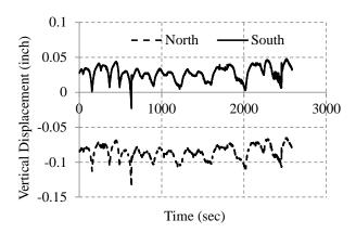
Figure 8-73. Axial displacement of the north and south vertical actuators
