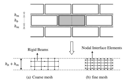
Figure 4-18. Two generated meshes for lattice model
