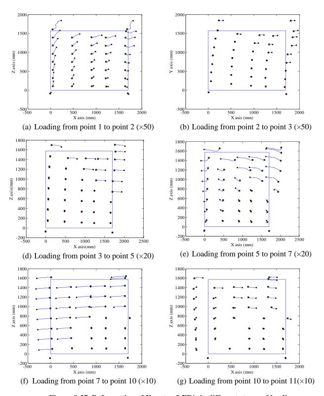
Figure 8-37. Deformation of Krypton LED's in different stages of loading
