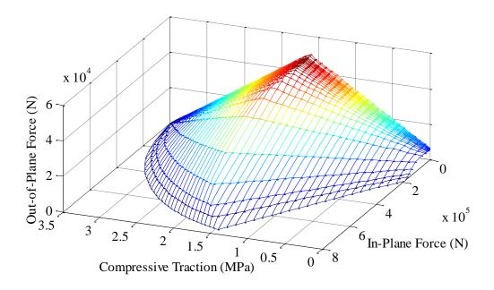
Figure 7-14. Interaction curve for a wide wall
