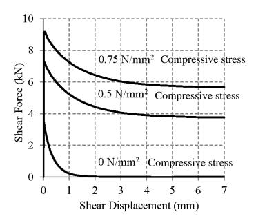
Figure 4-15. Response in shear with various compressive stresses
