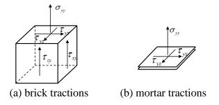
Figure 7-3. State of stress for brick and mortar
