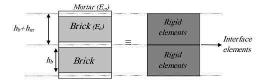
Figure 3-3. Calculating the stiffness of the interface elements
