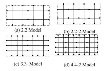
Figure 4-20. Different mesh sizes for modeling a brick
