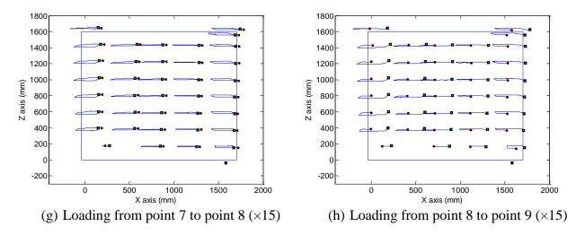
Figure 8-97. Deformation of the wall in different stages of loadings
