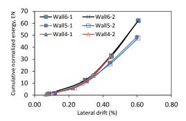
Figure 8-102 Variation of cumulative normalized dissipated energy
