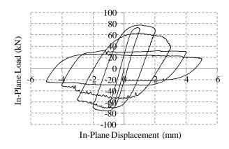
Figure 6-16. Load-Displacement for in-plane loading
