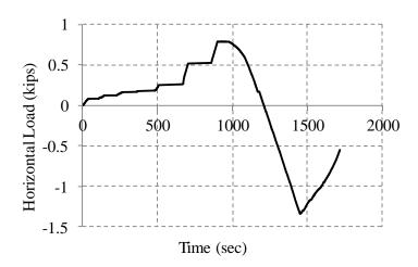
Figure 8-32. Loading protocol for wall 2
