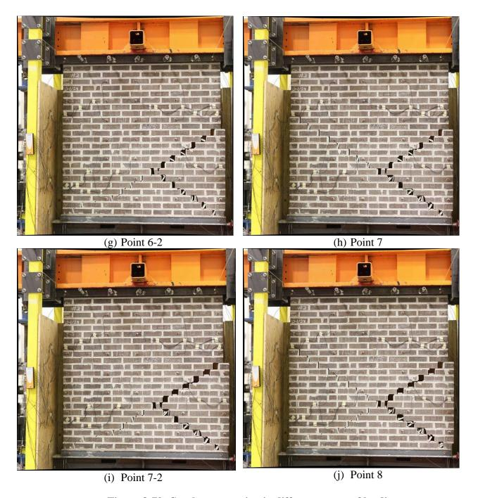
Figure 8-79. Crack propagation in different stages of loading
