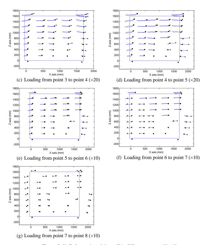
Figure 8-49. Deformation of the wall in different stages of loading
