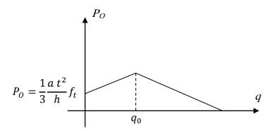
Figure 7-5. Interaction between tensile and compressive failure for OP loading (b) *Shear/tension regime*
