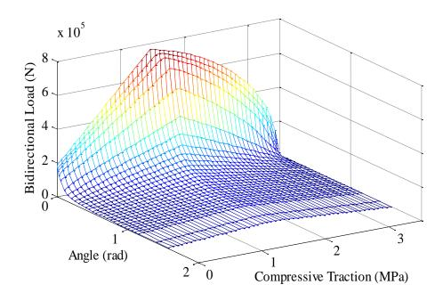
Figure 7-13. Variation of bidirectional load as angle and compressive traction change
