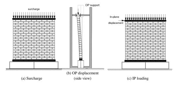
Figure 8-69. Combination of IP and OP loadings
