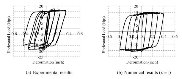
Figure 8-99. Comparison of the experimental and numerical load-displacement curves
