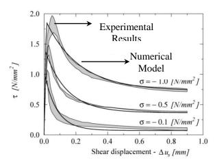
Figure 4-5. Shear behavior; experimental results by Pluijm [15] for different confinement levels, c=0.87 [N/mm²];  $tan\emptyset=1.01$ ;  $tan\emptyset_r=0.73$ ;  $G_f^{II}=0.058-0.13$  [N/mm]
