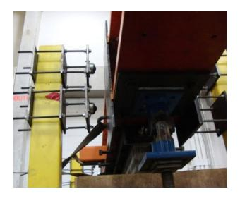
Figure 8-57. Support for large out-of-plane deformation of the wall
