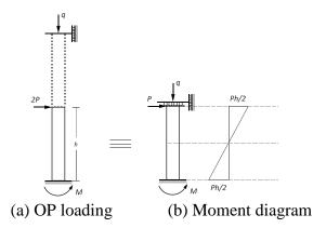
Figure 7-2. (a) Out-of-plane loading of URM shear walls (b) Moment diagram According to Figure 7-2, the maximum moment will take place at the supports. Equation (7-1) shows the distribution of the compressive/tensile stress at the face of supports.
