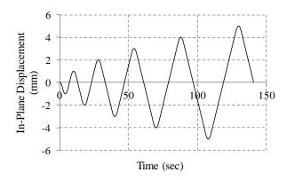
Figure 6-15. Displacement-time for the in-plane loading
