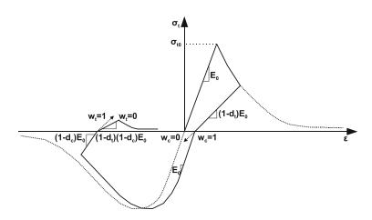
Figure 5-13. Concrete damage material model under uniaxial tension and compression test (Abaqus 2005)
