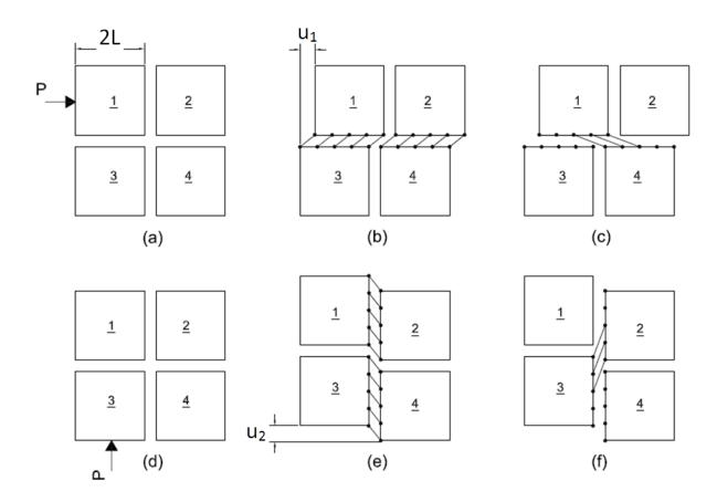
Figure 3-9. Updating contact length and detecting new contacts
