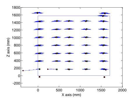
Figure 8-96. Deformation of the wall under cyclic loading ( $\times 10$ )
