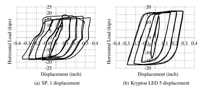
Figure 8-58. Load-displacement of wall 4
