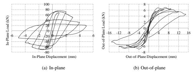
Figure 6-19. Load-displacement for IO:1/3 loading
