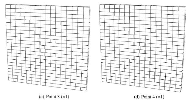
Figure 8-54. Numerical simulation of crack propagation in the wall
