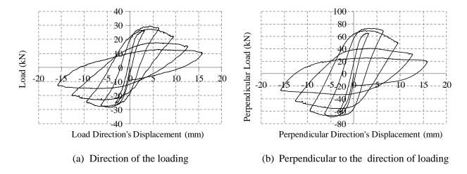
Figure 6-21. Load-Displacement curves for IO:1/3 model
