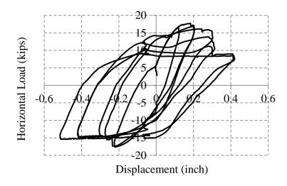
Figure 8-44. In-plane load-displacement curve of wall 3
