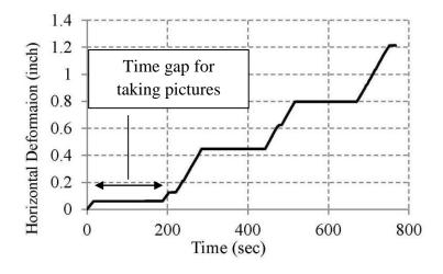
Figure 8-19. Loading protocol for wall 1
