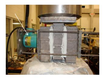
Figure 8-7. Test setup for measuring the shear properties
