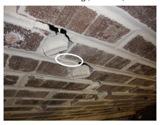
Figure 8-67. Out-of-plane gap in the joints at the end of the test
