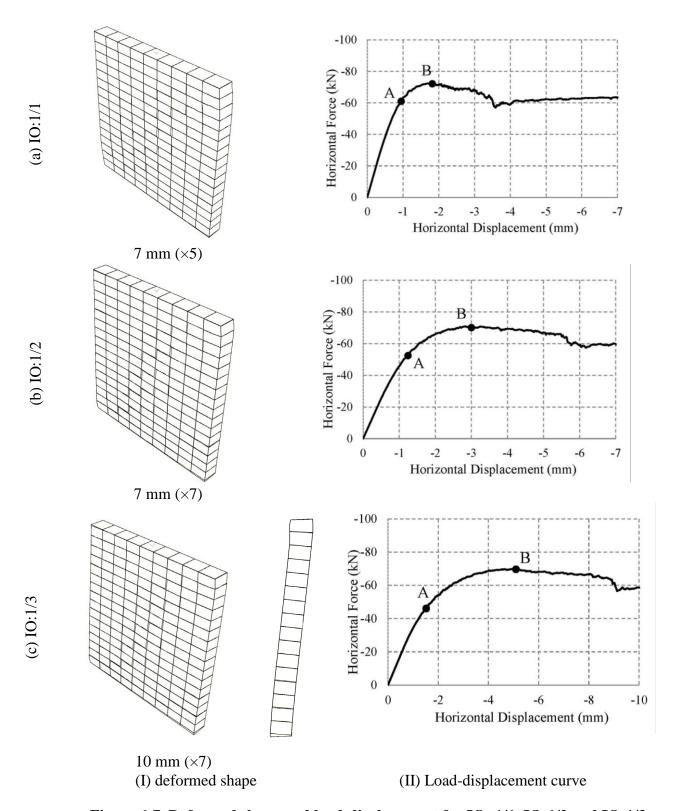
Figure 6-7. Deformed shape and load-displacement for IO: 1/1, IO:1/2 and IO:1/3
