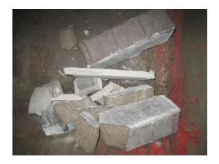
Figure 8-13. A damaged masonry prism after compression test
