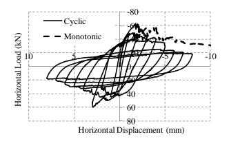
Figure 5-21. Cyclic load - displacement diagram for wall subjected to 30kN compressive load
