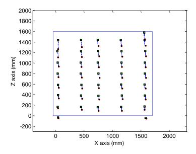
Figure 8-94. Deformation of the wall under the axial load (×300)
