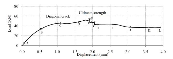
Figure 3-16. Load-displacement graph for J4D & J5D wall (Based on the model 4PB)
