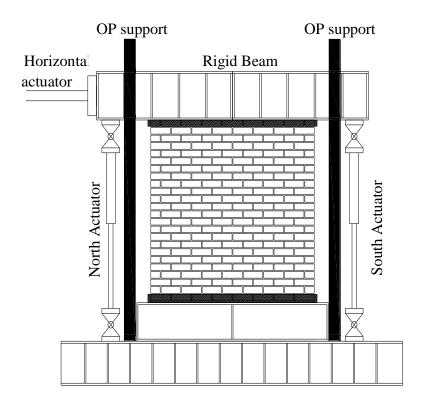
Figure 8-4. Test setup
