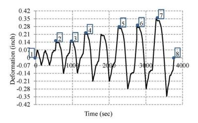
Figure 8-55. Loading protocol for wall 4
