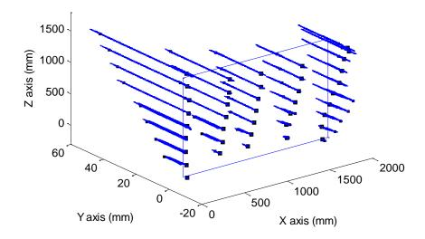
Figure 8-65. Three-dimensional deformation of the wall under cyclic loading (real scale)
