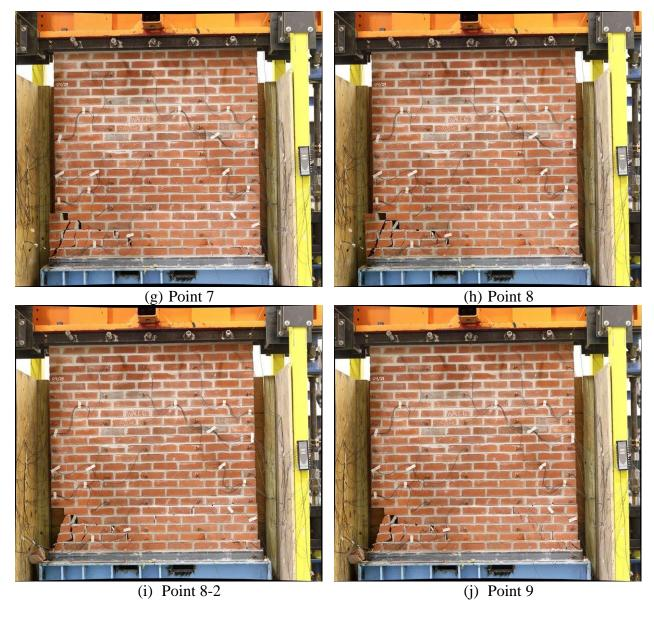
Figure 8-98. Crack propagation in different stages of loading
