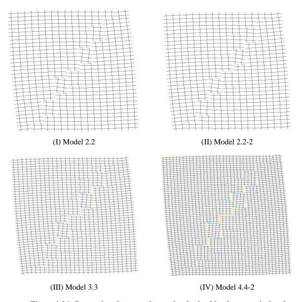
Figure 4-24. Comparison between the cracks obtained by the numerical and experimental models (J4D and J5D)
