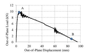
Figure 5-26. Load-displacement for out-of-plane direction loading
