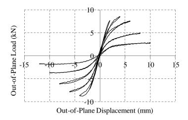
Figure 6-17. Load-Displacement for out-of-plane loading
