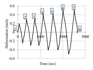
Figure 8-43. Cyclic loading protocol for the third wall
