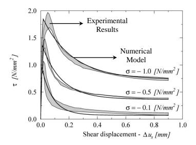
Figure 3-6. Shear behavior; experimental results by Pluijm [15] for different confinement levels, c=0.87 [N/mm<sup>2</sup>];  $tan\emptyset=1.01$ ;  $tan\emptyset_r=0.73$ ;  $G_f^I=0.058-0.13$  [N/mm]
