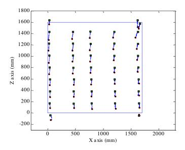
Figure 8-47. Deformation of the wall under the axial load (×500)
