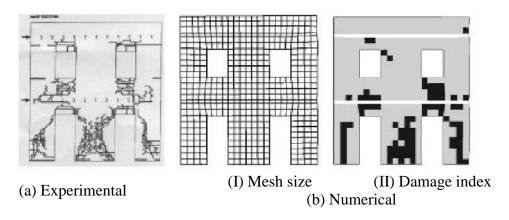
Figure 2-3 PAVIA wall: experimental crack pattern and damage index at the end of load history (damage areas in black color) (Karapitta et al. 2010)
