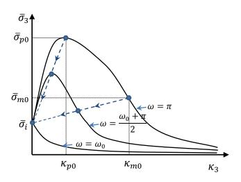
Figure 4-8. Modified Cap Plasticity Model for Interface elements
