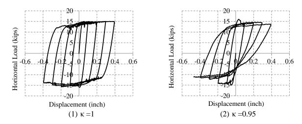
Figure 8-52. Cyclic load-displacement curves considering different values for stiffness degradation factor
