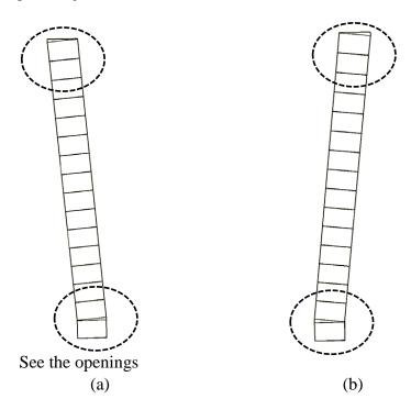
Figure 5-31. Deformed configuration of the wall under cyclic out-of-plane loading 5.9 Conclusion
