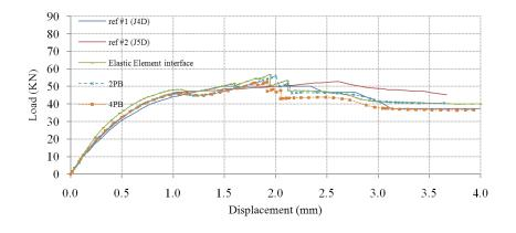
Figure 3-20. Load-displacement graph for J4D and J5D wall
