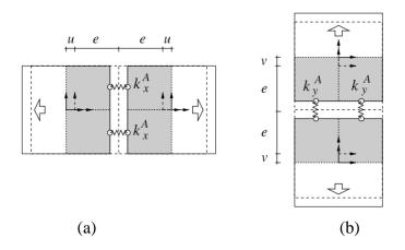
Figure 2-8. Rigid elements subjected to (a) horizontal and (b) vertical axial loading (Casolo and S. 2004)
