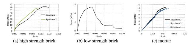
Figure 5-10. Stress-strain curves
