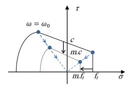
Figure 4-12. Isotropic Softening  $(0 \le m \le 1)$
