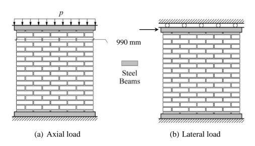
Figure 6-4. Step 1 and step 2 for applying the load (Lourenco 1996)
