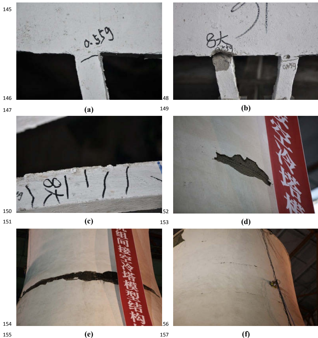
Fig. 5: Damage situation of support X shaped columns and hyperboloid shell
