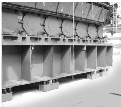
142 143 Figure 2: Spring supported diesel engine
