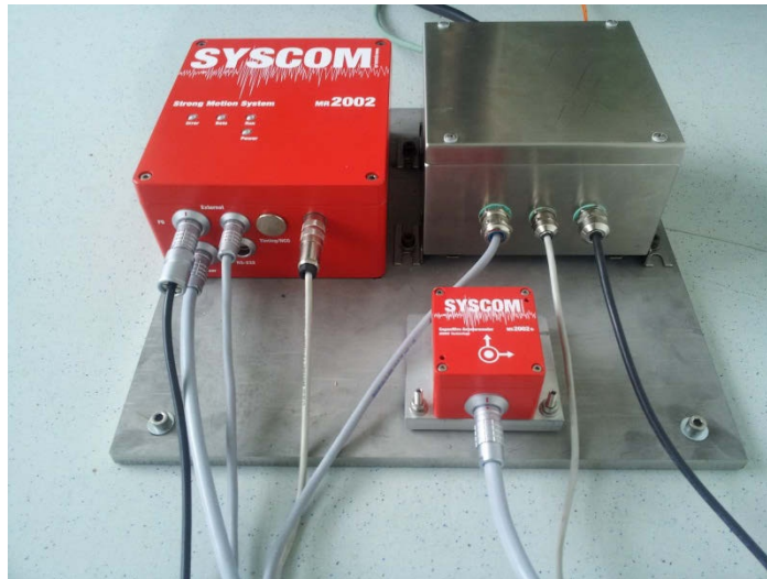
113 114 Figure 3: Strong motion recorder (MR2002), Accelerometer (MS2002) and stainless steel 115 junction box mounted on a platform
