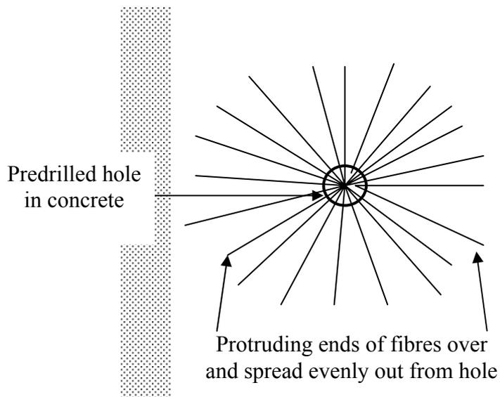
Fig. 7-8: Top view of the anchor system.
