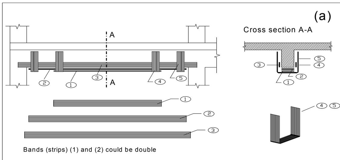
Fig. 7-1: Flexural reinforcement with possible shear anchorages.
