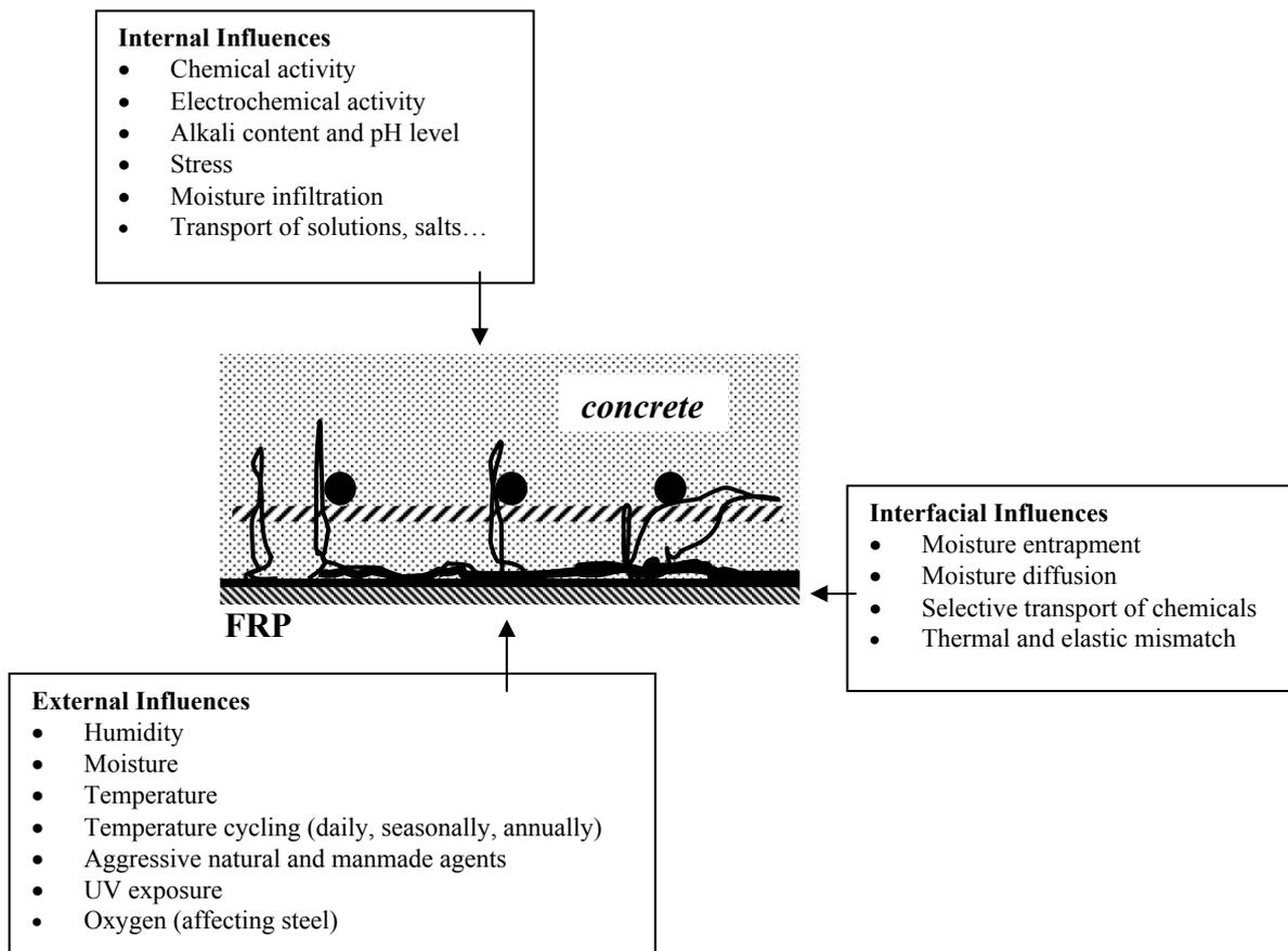
Fig. 9-1: FRP system level interactions.
