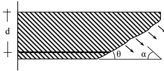
Fig. 5-5: Contribution of FRP to shear capacity.
