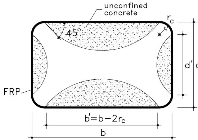
Fig. 6-8: Effectively confined core for non-circular sections.
