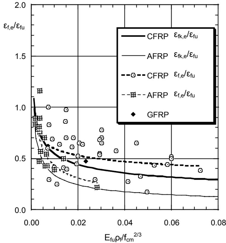
Fig. 5-7: Normalized FRP strain in terms of  $E_{fu}\rho_f/f_{cm}^{2/3}$  – shear failure combined with or followed by FRP fracture.
