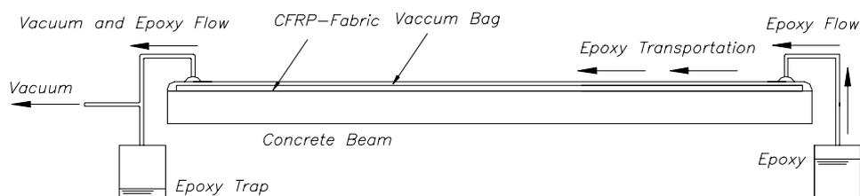
Fig. 2-10: Strengthening with vacuum injection system (Täljsten and Elfgren 2000).
