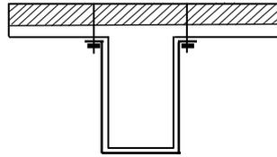
Fig. 7-4: Alternative anchorage in the compression zone.
