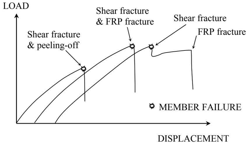
Fig. 5-4: Schematic illustration of shear failure response.
