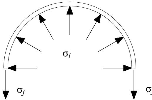
Fig. 6-3: Lateral confining pressure exerted by the jacket.
