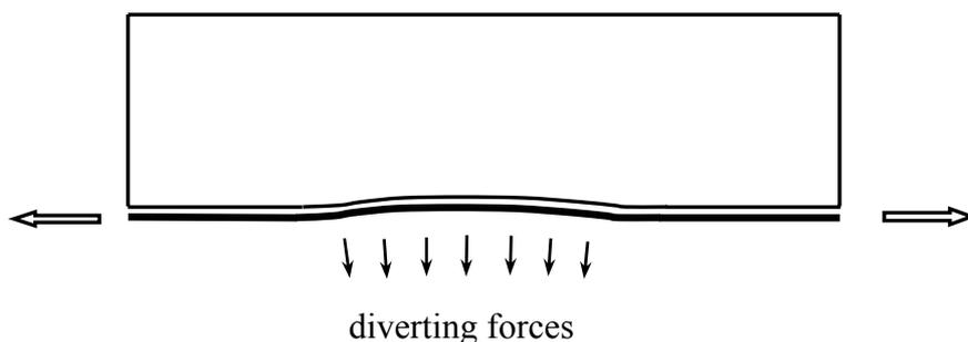
Fig. 4-14: Peeling-off caused by unevenness of concrete surface.
