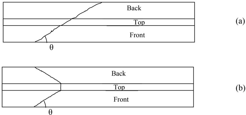
Fig. 5-9: (a) Torsional and (b) shear cracking.
