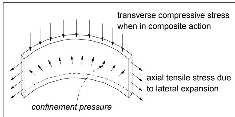
Fig. 6-2: Triaxial state of stress in FRP jackets.
