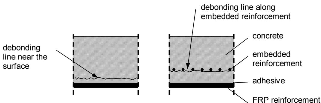
Fig. 4-4: Different debonding lines in the concrete.
