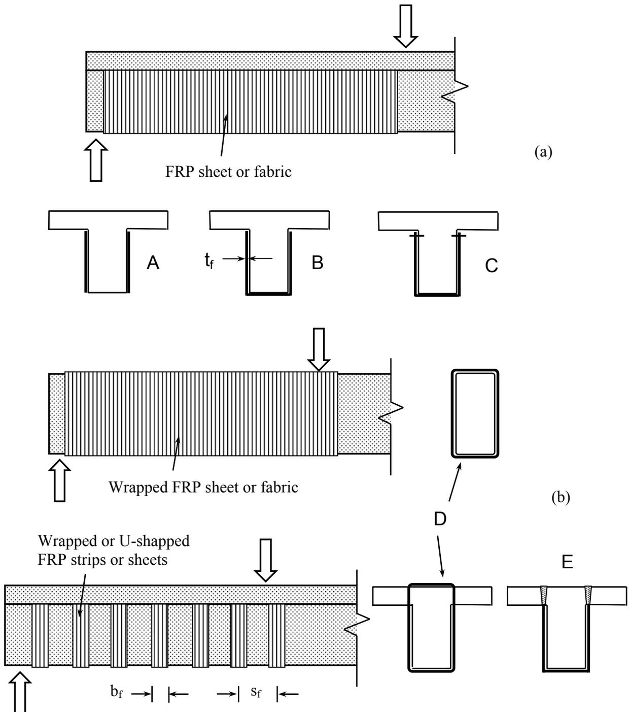
Fig. 5-2: Schematic illustration of reinforced concrete element strengthened in shear with FRP: (a) FRP sheets or fabrics bonded to the web; (b) wrapped or U-shaped FRP (the concept shown in D is applicable to both beams and columns).
