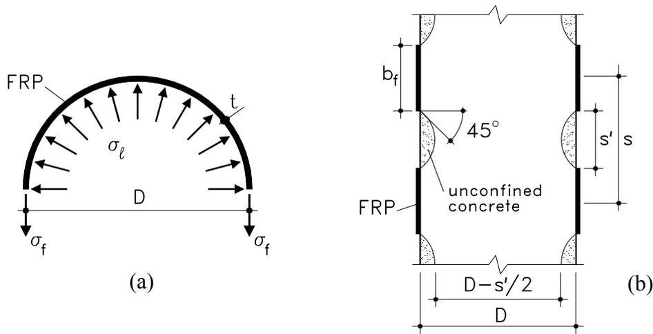
Fig. 6-7: Confining pressure exerted by the FRP.
