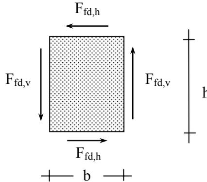
Fig. 5-10: Forces carried by the FRP reinforcement.
