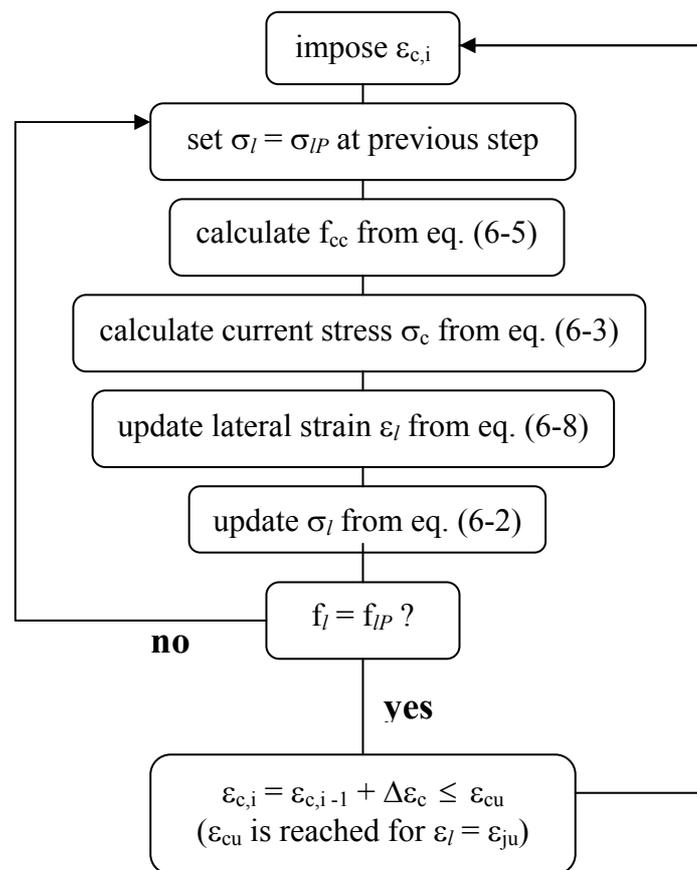
Fig. 6-4: Iterative procedure of Spoelstra and Monti (1999) model.
