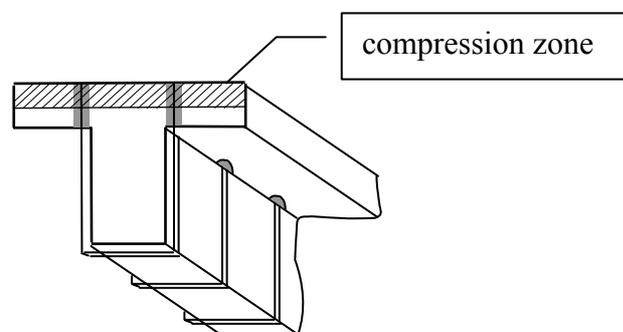
Fig. 7-3: Anchorage in the compression zone.
