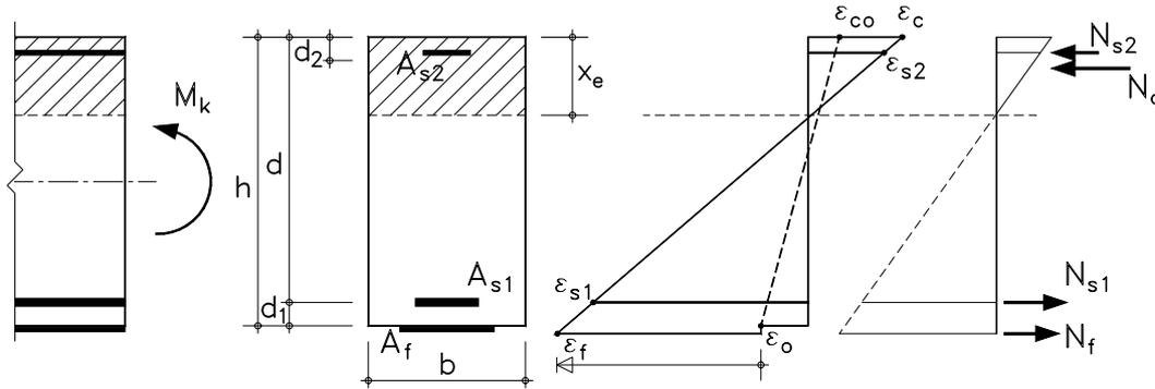
Fig. 4-15: Linear elastic analysis of cracked section.
